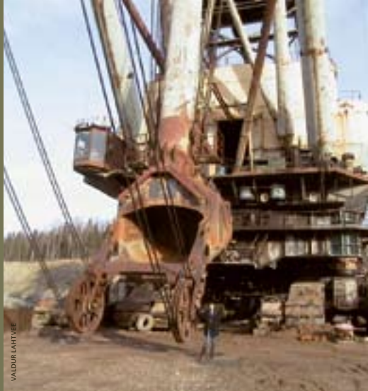
A 'walking excavator' at Narva, Estonia. The Narva complex consists of the world's two largest oil shale-fired thermal power plants.
